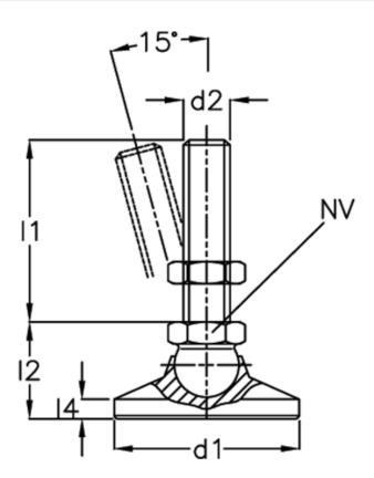
A/F = 24 d1 = 60 d2 = 24 l1 = 138 l2 = l4 = -Static load (N) = 30 Weight in (g) = 630
